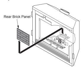
Figure 43 - Installing Rear Brick Panel
